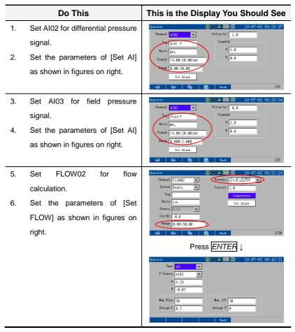
The instrument provides flow totalizer, which supports up to 16 channels totalizer and displays the logs of per month, per day, per hour and also customized. After applying the correct totalizer settings, it will calculate the total flow, which is measured through any selected signal.
