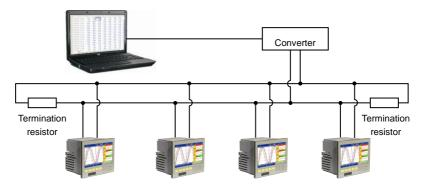
Figure 2-12 RS-485 communication between computer and several instruments
