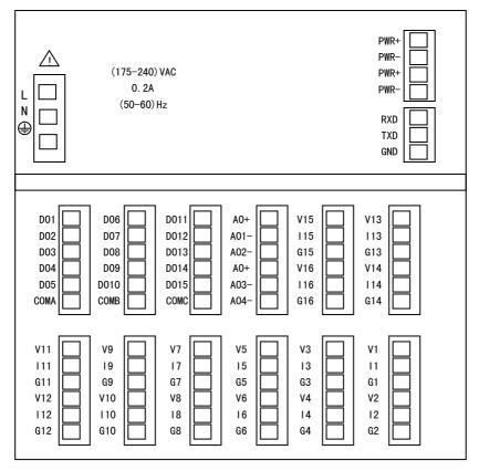
Figure 2-4 Terminal arrangement
