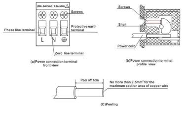
Figure 2-5 Power supply connection
