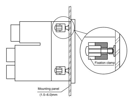
Figure 2-2 Diagram for installation
