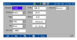
Figure 6-1 [Control Loop] Display
