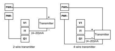
Figure 2-9 Transmitter power supply connection
