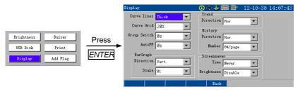
Figure 4-6 Display Setup
