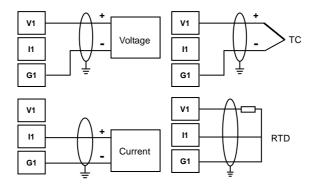
Figure 2-6 Analog input connection
